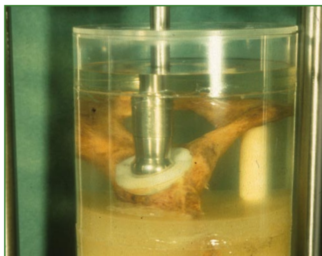
Fig. 3 Setup of the adhesion test with the coated RM cup in a pelvis specimen. The cadaver pelvis is embedded in PMMA and the whole setup is dipped into a formaldehyde solution and kept at 23°C.
